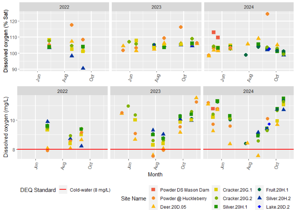
Chart 2. Observed dissolved oxygen saturation (top, in %) and concentrations (bottom, in mg/L) for the Upper Powder watershed monitoring sites over the 2022-2024 period. Cool-water standard (red line) highlighted.
