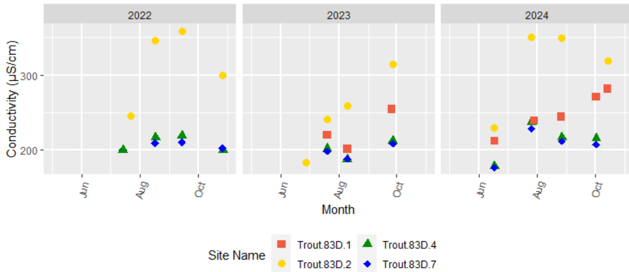
Chart 45. Observed conductivity measurements (in \mu\text{S}/\text{cm} ) for the Trout Creek monitoring sites over the 2022-2024 period.
