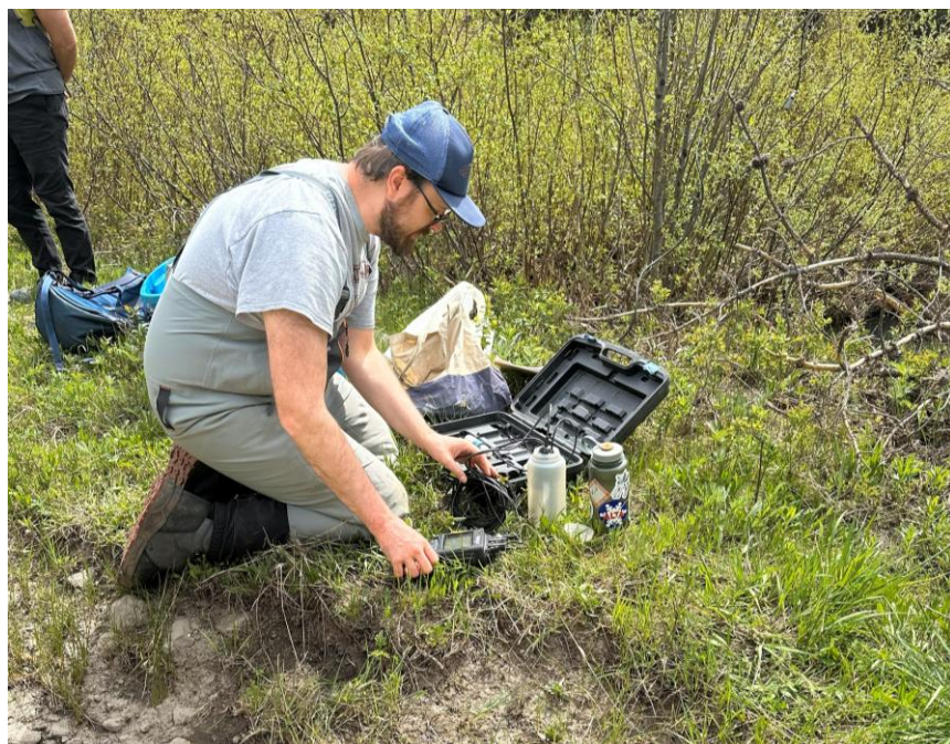
Figure 8. Grab sample monitoring near a monitoring site using the Orion A329 and Hach 2100Q Turbidimeter
